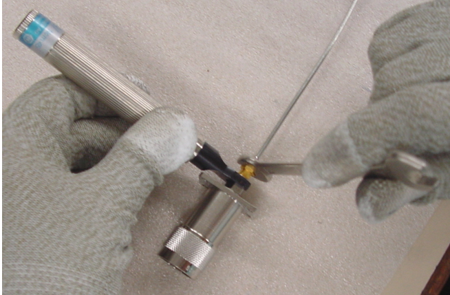
Fig. 3-10 Connect the coax assy (item 10) to the N-SMA connector (item 07) using a torque wrench
